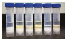
Samples after centrifuging the QuEChERS salt extracts, from left to right; blank, butter, cheese, egg, milk and fish
